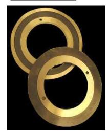
SHB manufacture Gear Deburring Cutters to remove burrs formed during teeth cutting and chamfering operation. These cutters are used in conjunction with Gear Chamfering Cutters. Material used is mainly HSS M-2. Gear Deburring Cutters for Samputernsilli Machines can be manufactured in standard form as well as to the specific requirements of the customer.
