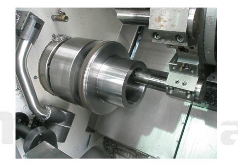
Turning is the process whereby a single point cutting tool is parallel to the surface. It can be done manually, in a traditional form of lathe, which frequently requires continuous supervision by the operator, or by using a computer controlled and automated lathe which does not. This type of machine tool is referred to as having computer numerical control, better known as CNC. and is commonly used with many other types of machine tool besides the lathe.
