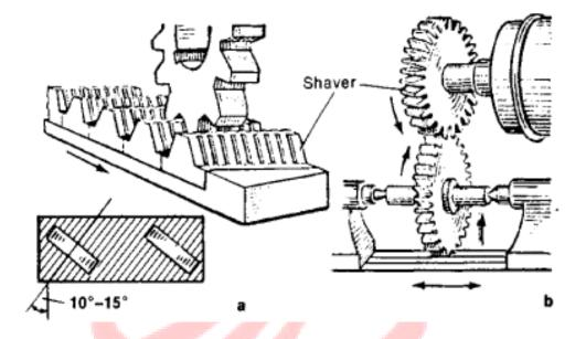
Gear shaving is basically a finishing operation. This takes place after the operations of roughing with a hob or cutting with a shaper cutter is over. The Shaving process consists of the removal of tiny particles of metal from a gear teeth's working surface. Gear shaving produces fine hair like chips. The cutter comes in the form of helical gear. It has special serrations in the flank area of gear teeth. These serrations act as the cutting edges.
