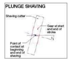
In this method there is no worktable translation. Instead there takes place a radial feed of the work piece against the tool that is used as shaving cutter. Plunge shaving is particularly good for shaving of shoulder gear.
