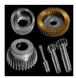
SHB Manufacture Gear Shaping Cutters in Module, DP and CP series. Spur as well as Helical Shaper Cutters can be supplied in Disc, Hub and Shank Type Varieties. Material used is generally AISI M35 Grade and accuracies are as per DIN-1829 Standard Class 'AA' and Class 'A'. Profile modifications including Chamfer, Semi-Topping, Topping , Protuberance, Flat or Fillet Root can be provided.
