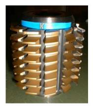
The hob is the cutter used to cut the teeth into the work piece. It is cylindrical in shape with helical cutting teeth. These teeth have grooves that run the length of the hob, which aid in cutting and chip removal. There are also special hobs designed for special gears such as the spline and sprocket gears.
