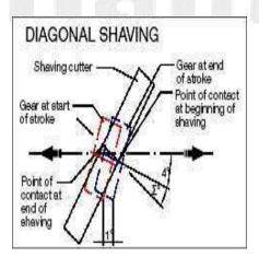
Here the gear selected for shaving reciprocates obliquely in direction to its own axis. The gear and the tool are made to stay in a mesh. The diagonal angle can be got by positioning of the work piece table in an oblique manner or by the process of interpolating of the two machine axes. As with each reciprocation, there is a radial feeding of the shaving cutter. This is described in the diagram.
