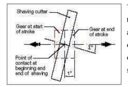
The gear that is shaved reciprocates in the direction of its own axis. The tool and the gear are in mesh. With each step of reciprocation, there is an occurrence of small quantity of radial feeding of the shaving cutter.
