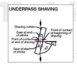
Underpass shaving is primarily identical to diagonal shaving with a small variation in the form of a diagonal angle of 90 degrees. In underpass shaving no axial table reciprocation takes place. In its place, the work piece reciprocates at right angles to its own axis.
