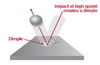
Shot Blasting is the process after Heat treatment in which remove the product darkness which occurs in heat treatment process . In this Process 52 to 60 HRC hardness stainless steel small particles strike on product.
